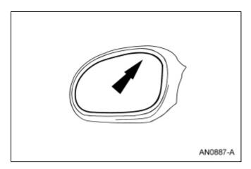
2. WARNING: Place a shop towel between the hands and the exterior mirror glass for protection in case of glass breakage during mirror service. Failure to follow this instruction may result in serious personal injury.
